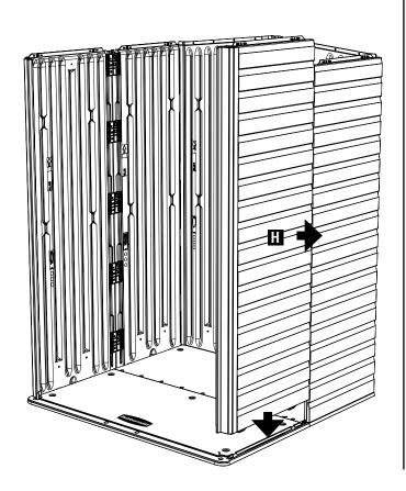
Using a screwdriver, punch out the screw holes on the top of the **Front Right Side (H)** 2 places.
